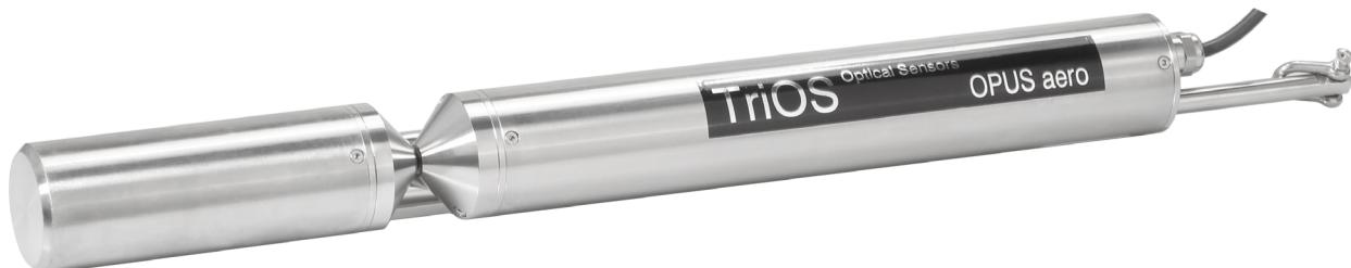
OPUS aero is the new generation of spectral sensors for online measurement of nitrate and nitrite in wastewater aeration tank. By analyzing a complete spectrum, OPUS aero is able to provide reliable readings for either NO<sub>3</sub>-N only or NO<sub>3</sub>-N and NO<sub>2</sub>-N, depending on the calibration.
