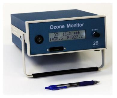
The 2B Technologies Model 202 Ozone Monitor<sup>™</sup> is designed to enable accurate and precise measurements of ozone ranging from low ppb (precision of ~1.5 ppb) up to 250,000 ppb (250 ppm) based on the well-established technique of absorption of UV light at 254 nm. The Model 202 Ozone Monitor<sup>™</sup> is lightweight (5.5 lb, 2.5 kg) and has a low power consumption (12V DC, 0.60 amp, ~7.2 watt) relative to conventional instruments and is therefore well suited for applications such as:
